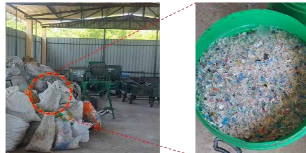
Figure 21: Storage of shredded flexible plastic waste at RRC
