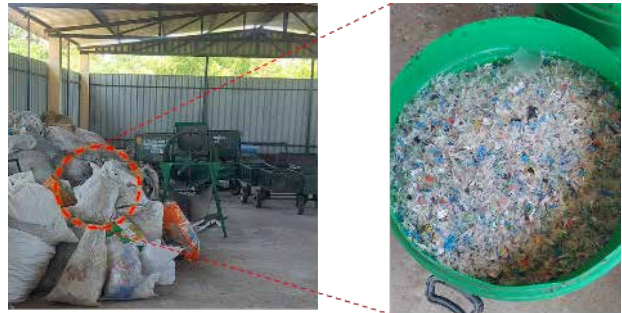
Figure 21: Storage of shredded flexible plastic waste at RCC
